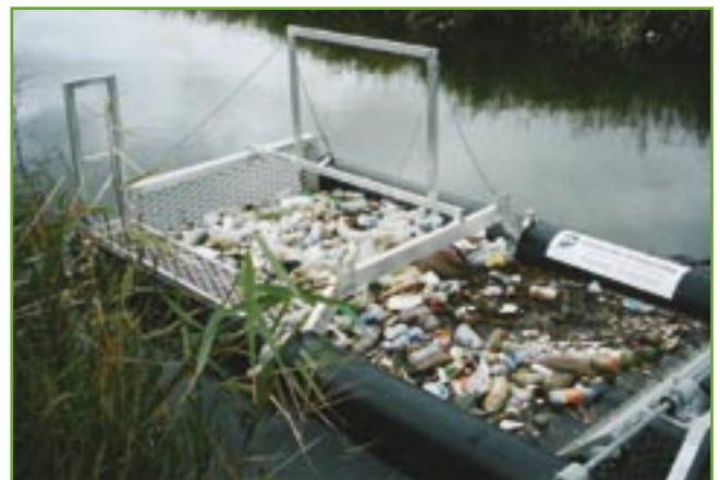
A Bandalong Litter Trap successfully protecting the environment.
