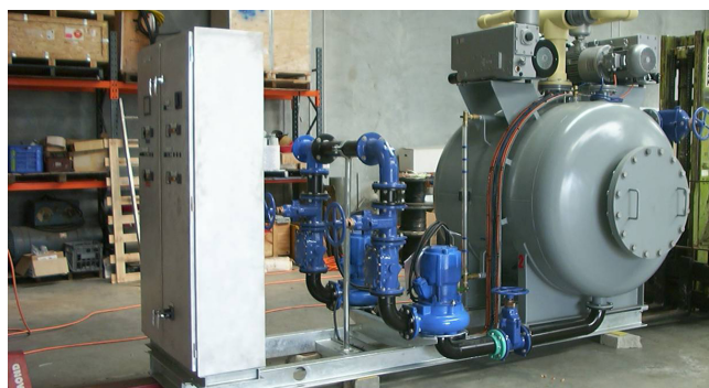
FLOVAC VACUUM STATION: A compact system delivered pre-assembled.
